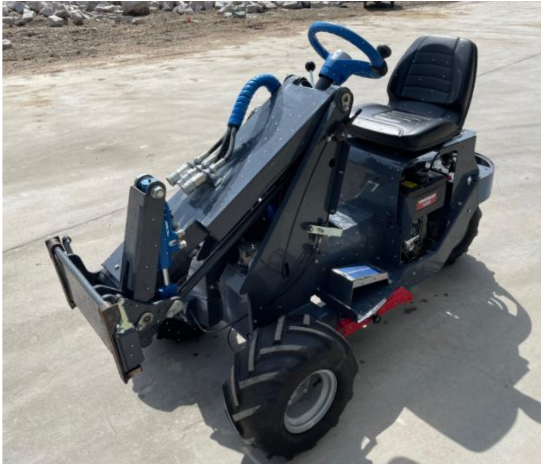
Mini wheel loader H130 Picture (hydrostatic model )
