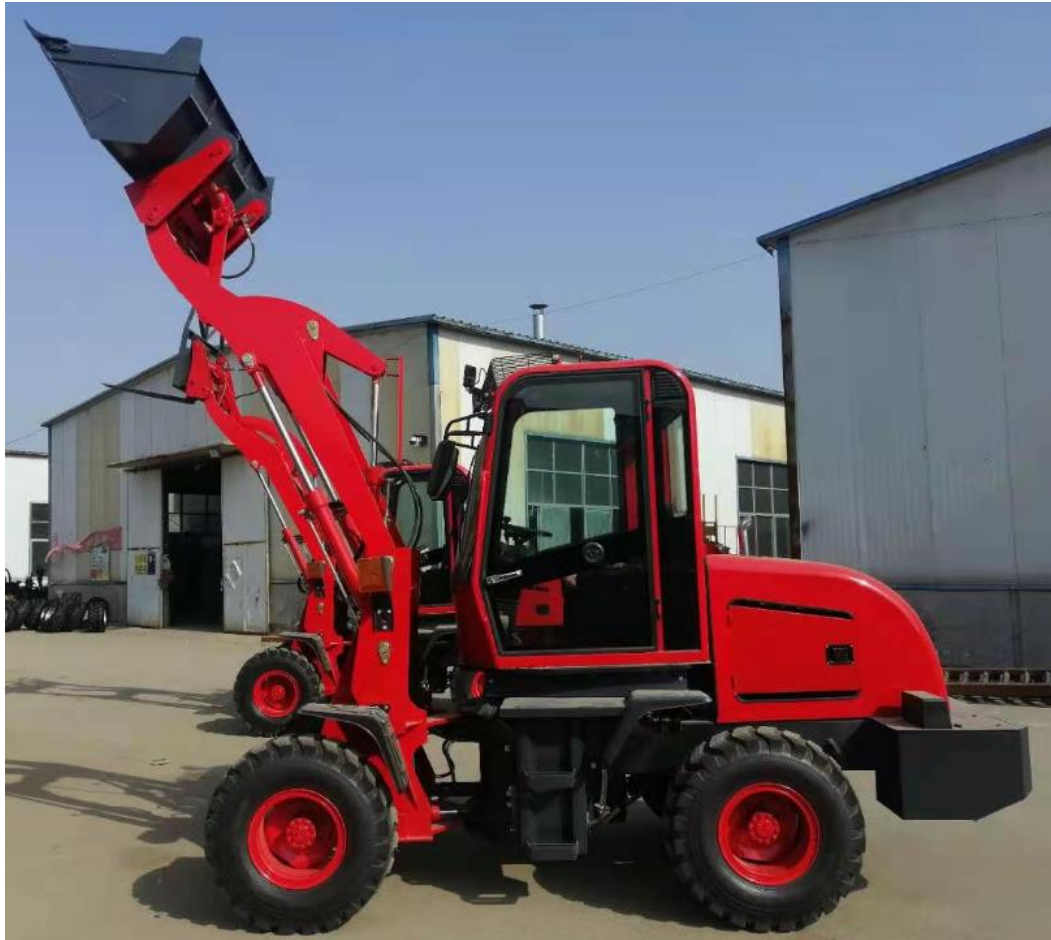
Mini wheel loader ZL15 Picture (traditional transmission )
