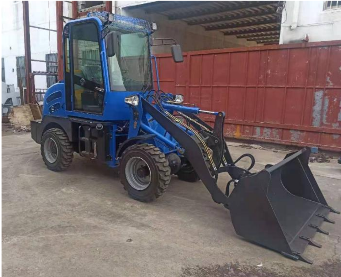
Mini wheel loader ZL12 Picture (traditional transmission )
