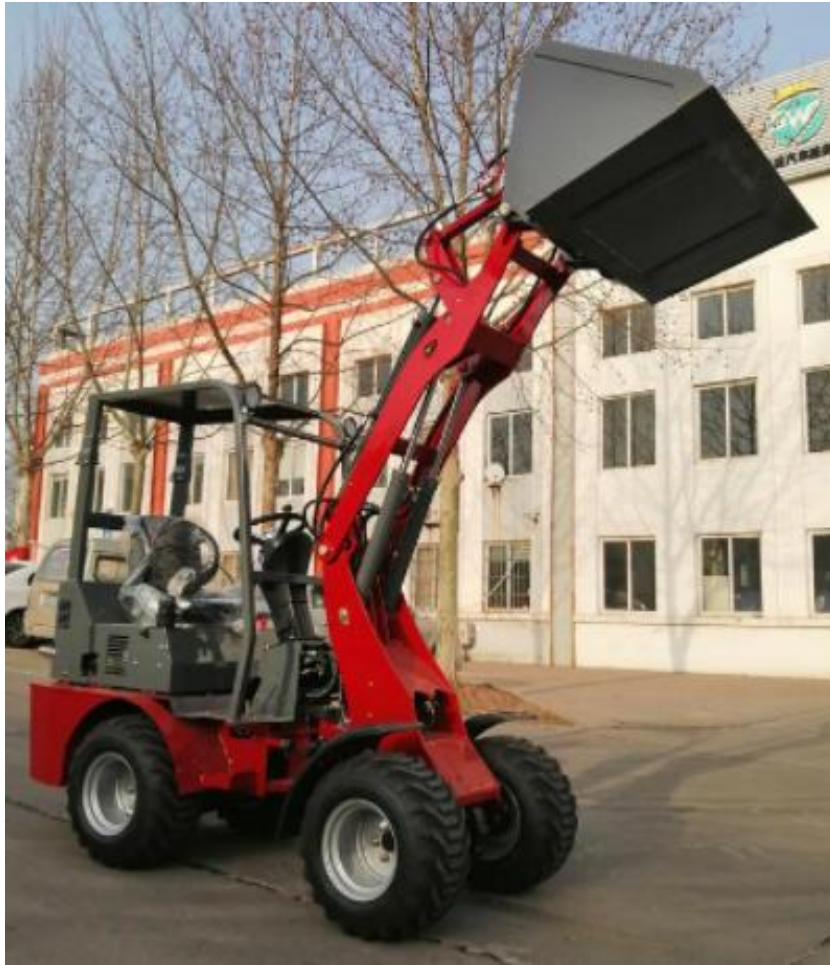
Mini wheel loader D25 Picture (hydrostatic model )
